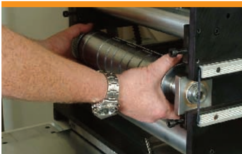
BAR's machines feature a horizontal loading die system
