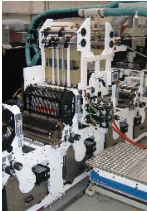
Omet hologram insetting unit in-line on a Varyflex
