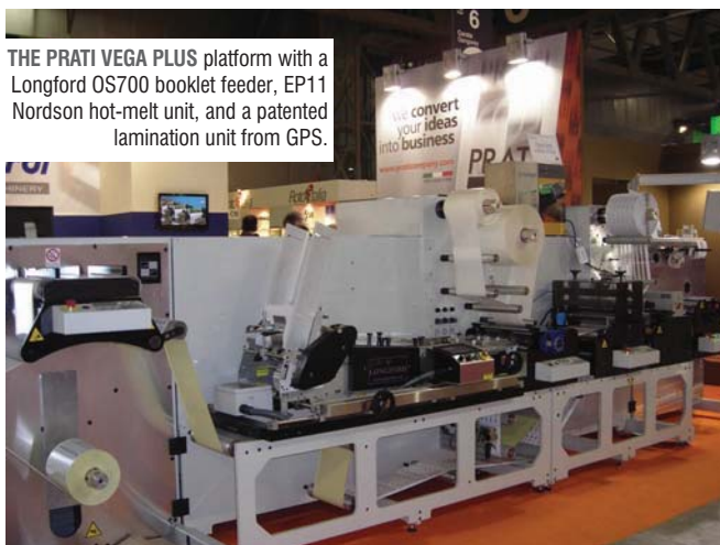
THE LAMINATION STATION on Prati's off-line booklet making machine can be adjusted so the booklet label fits exactly the shape of the container.
