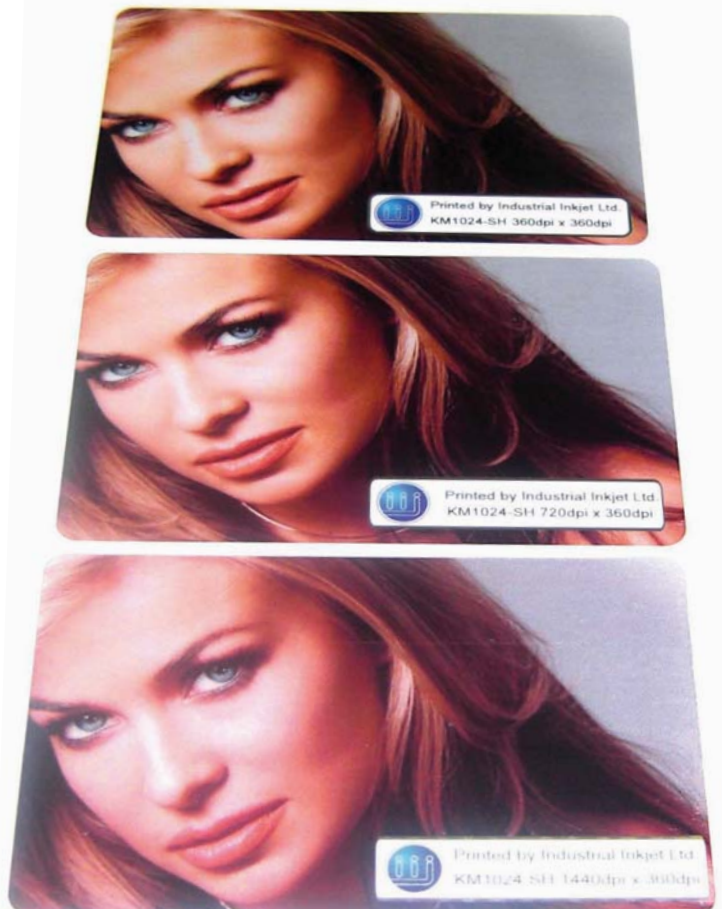
TOP TO BOTTOM: 360 x 360dpi, 720 x 360dpi, 1440 x 360dpi. All printed on KM1024 system
