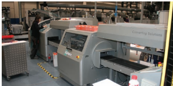
(THREE IMAGES RIGHT, TOP TO BOTTOM) The Label CS produces counted strip stacks directly from the reel in one process, including strip cutting, punching and automatic banding and palletizing
